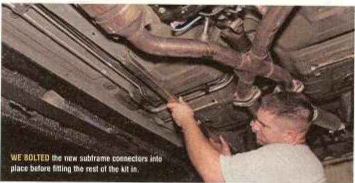
KENNY BROWN sent out its Extreme Matrix Kit, which includes subframe connectors, jacking rails, and matrix bars to connect the two. Brown also sent out its strut lower brace and rear shock lower brace to stiffen the rest of the chassis.
