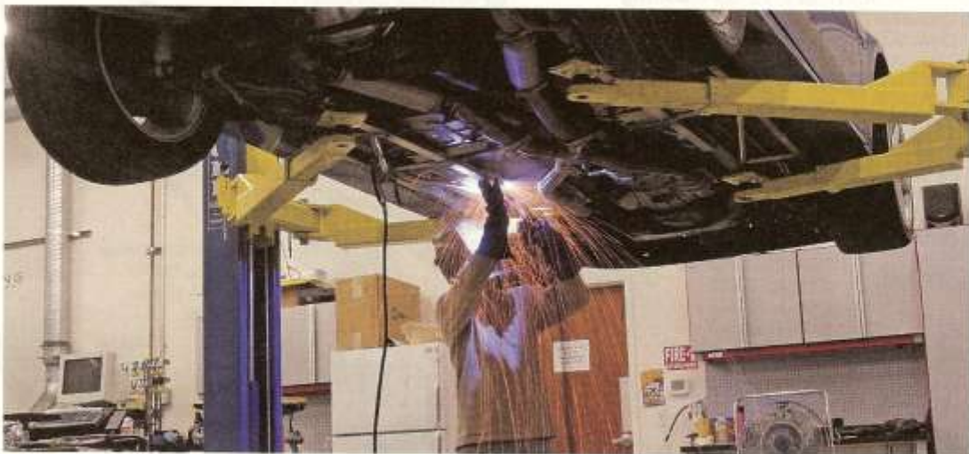
MM&FF'S NEWEST associate editor, Marc Christ, dug in and started welding our chassis support system.
